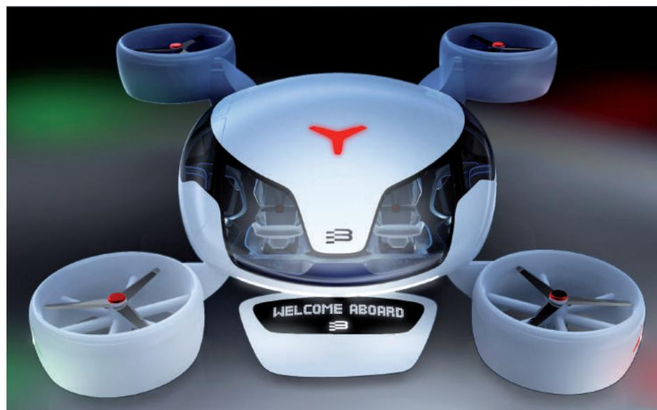
A cuttlefish-bone shaped body surrounded by four propulsors, each of which has two electric motors, at its furthest points. The Russian VTOL developer chose Italdesign to design the passenger compartment and the glass surfaces of its first aircraft capable of performing take-off and landing in wholly electric mode.
